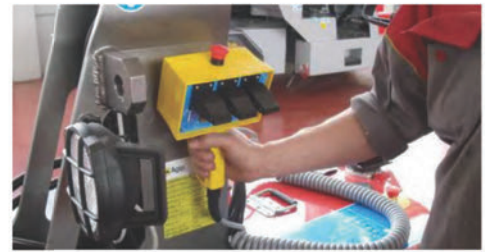
Fully proportional, wired remote for the crane functions.
