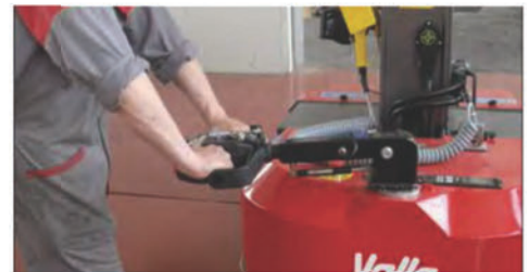
180 degree power assisted steering for maximum maneuverability.
