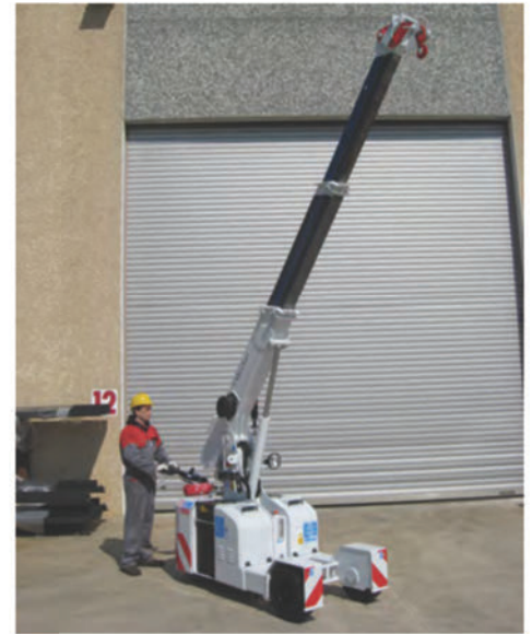
3 section hydraulic telescopic boom.
