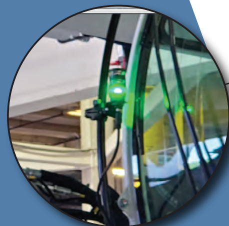
- LMI Utilization Light Tower Notifies personal of Crane Condition
