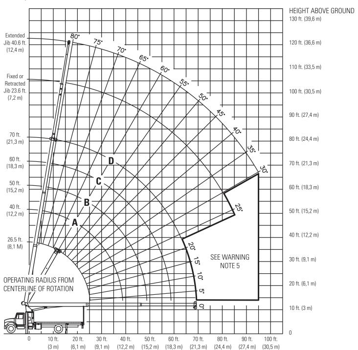
Lifting Capacities 3-section Boom 26.5 ft. - 70 ft. Jib 23.6 ft. - 40.6 ft.
